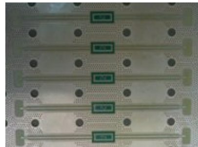
Figure 3 - Filters soldered in a wave-guide test board
