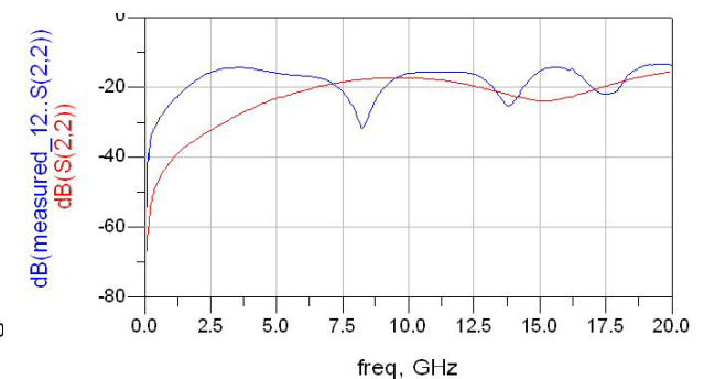
Reverse Return Loss (S11) plot of simulated and measured
