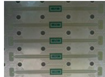
Figure 3 - Filters soldered in a wave-guide test board
