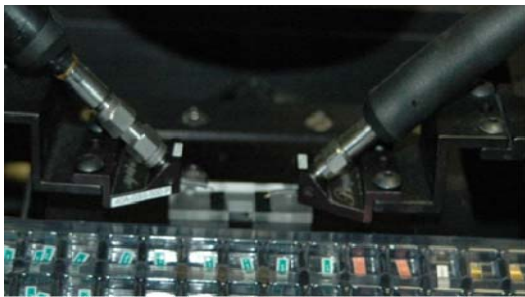
Figure 1 - measurement setup with G-S-G probes
