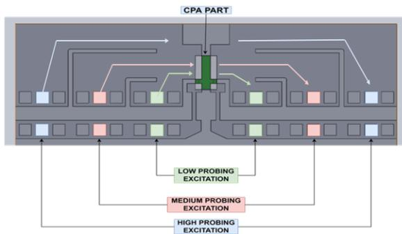
Figure 1. CPA Part on Test Board with Excitation Locations
