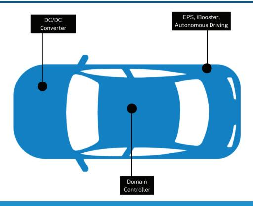
There are a variety of CSS applications within the automotive Advanced Driver-Assistance Systems (ADAS). This includes electronic power steering, also known as EPS, to an electromechanical brake booster, and autonomous driving. Other
